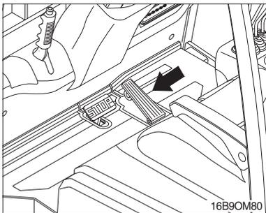
(1) This pedal is used to vary running speed, which depends upon how far the pedal is depressed.
