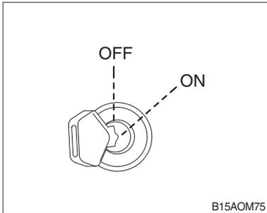
(1) Power is supplied to the control circuit through this switch, which is placed on OFF → ON clockwise.
