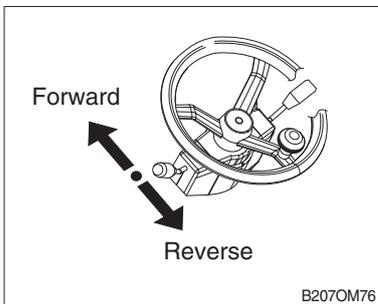
(1) This lever serves to make forward/backward directional changes. For the forward directions, place the lever on the FORWARD position.
