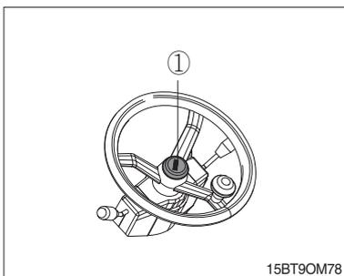
(1) When the button (①) is pressed, the horn will sound.
