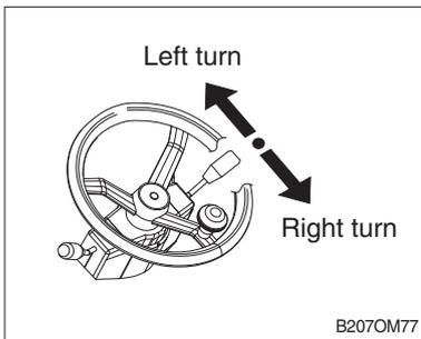
(1) When making a left or right turn, use this switch to flash the flash lamp to indicate which direction the vehicle is turning to.
