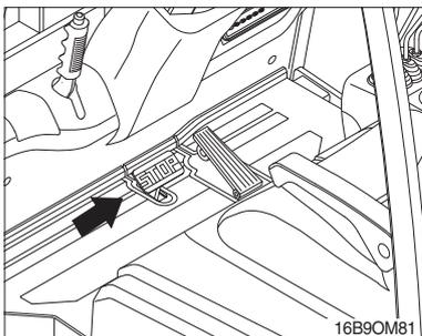
(1) When this pedal is depressed, the vehicle is braked, while the braking lamps attached on the rear light.
