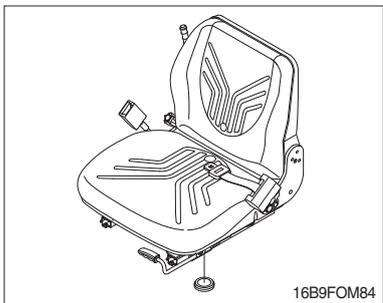
(1) This switch is closed automatically when an operator sits down on the seat.
