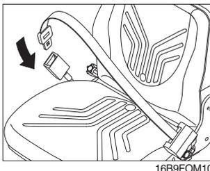
(1) Buckling up. Be sure that you put on the seat belt. Connect and adjust the seat belt strap to a snug, comfortable position.
